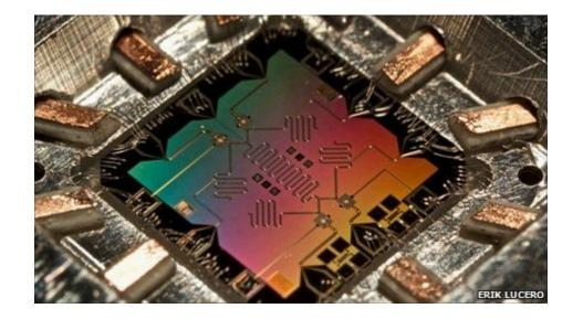
Here is a picture of a quantum processor using transmon superconducting qubits.
